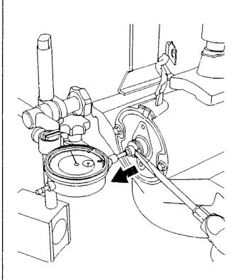
Assembling bearing end plate
